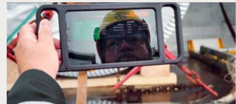
2. The secured cargo is photographed, and an AI-powered app verifies if the load has been properly secured.
